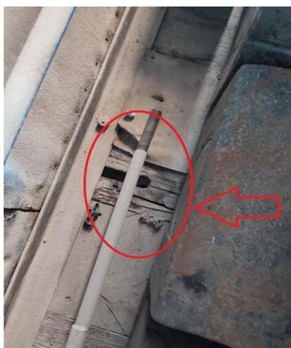
Fig. 5. Aging of the wooden floor of the weighing wagon model VPV-640
