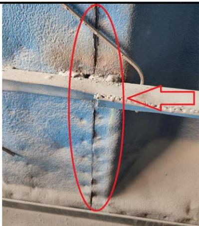
Fig. 3. Crack in the inner wall of the body of the weighing wagon model VPV-640 due to external impact
