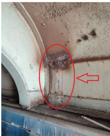
Fig. 4. Crack in the roof part of the body of the weighing wagon model VPV-640 due to the weight load of exemplary weights
